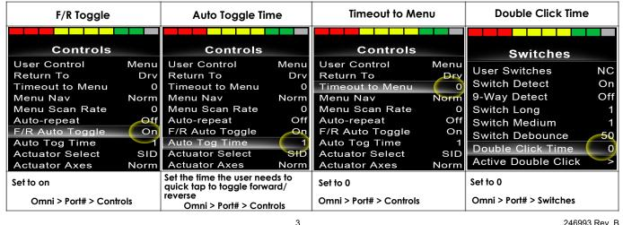
**Setup 2** - Short user switch to toggle forward and reverse; double click user switch to activate mode function a. Ensure power chair port is set for 3 direction driving.
