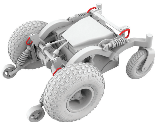
Figure 5.2c Frontier V4 lifting points
