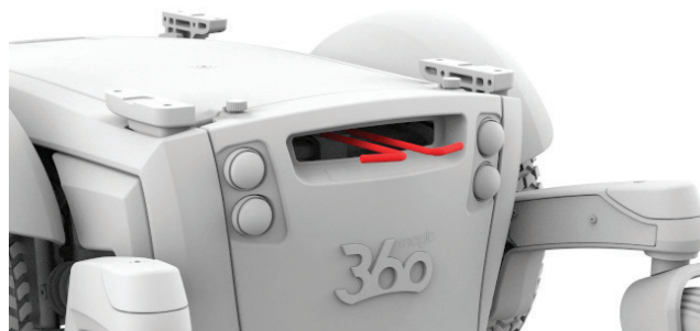
Figure 4.4b Magic 360 brake levers released
