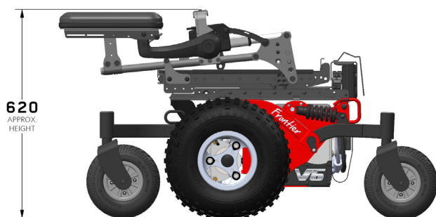
Figure 4.3c Frontier V6 and V4 Fold Forward height
