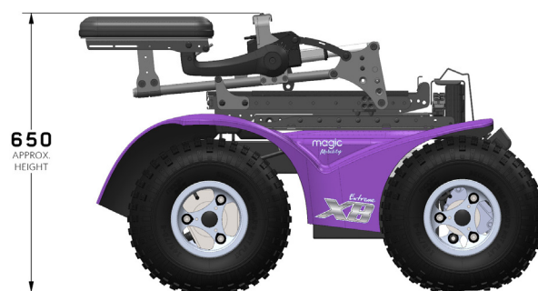
Figure 4.3d Extreme X8 Fold Forward height
